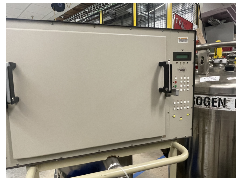
Figure 2: EC13 environmental chamber with front experimental setup enclosed
