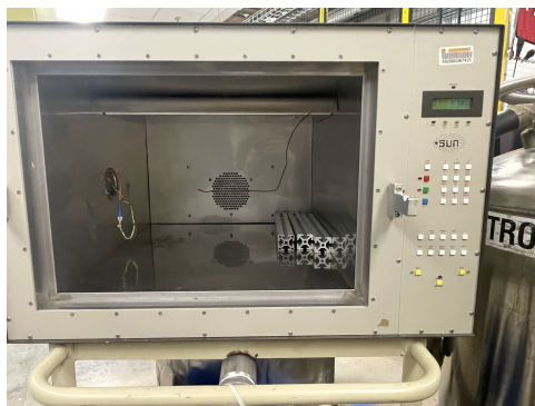
Figure 1: Experimental setup internal to the EC13 environmental chamber
